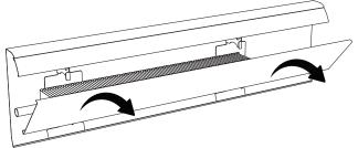
3. Remove any existing damper sections.
